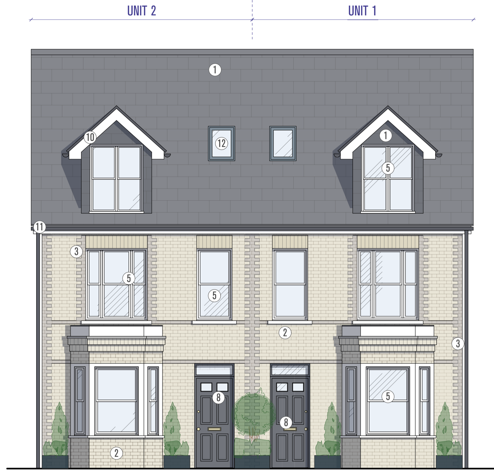
Elevation A-A (Front; 80 Croydon Road)
